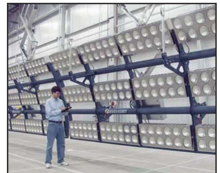
GM Milford Proving Grounds Rollover Lighting System – 1728 kW Tungsten
