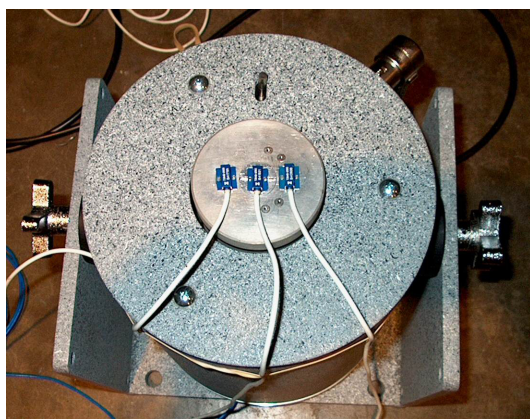
CAL 50 exciter with 3 PR DUTs mounted
