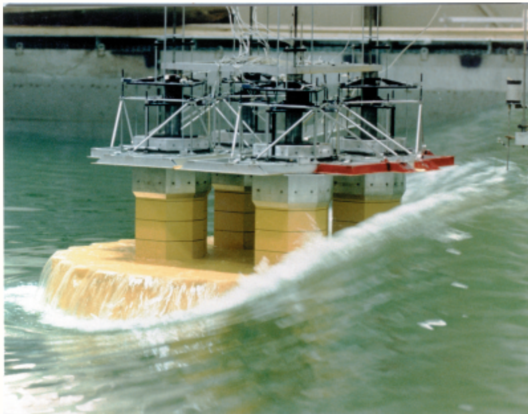
Interaction of extreme waves with Hibernia GBS platform
