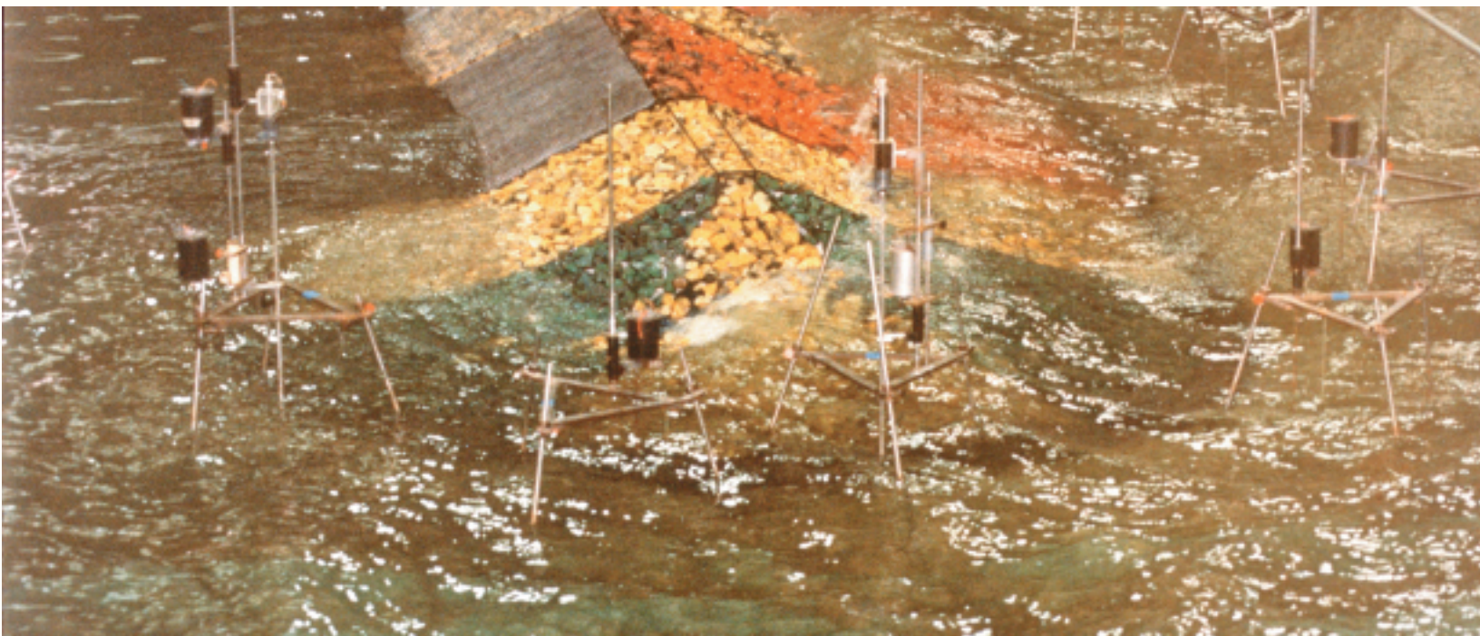
Stability of a breakwater head under multidirectional waves
